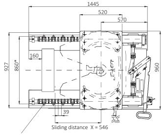
\* recommended hole pattern 10 x countersink on each side for countersunk bolts M14
