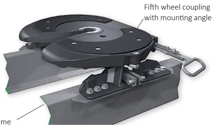
The fifth wheel coupling is built onto either the frame or sub-frame of the tractor. The JOST mounting instructions for fifth wheel couplings and mounting plates, as well as the respective mounting instructions supplied by the vehicle manufacturer must be observed when mounting or converting equipment.
