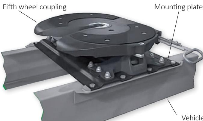
The fifth wheel coupling is fixed to the tractor frame by means of a mounting plate. Various mounting plate and fifth wheel mounting heights are available to facilitate an accurate match between the height of the fifth wheel and existing trailer systems.
