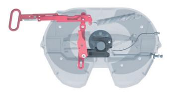
The tappets in the insertion area ensure that the king pin is guided accurately into the fifth wheel coupling.
