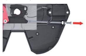
Wearing ring easy to replace without dismantling the fifth wheel coupling.
